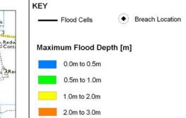
Hydraulic modelling has been undertaken using 2-D hydraulic nodelling software MIKE21-HDFM (ver. 2009), to assess the effect of breaches at specified points and/or overtopping of defences.
