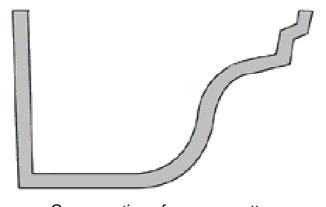
Cross section of an ogee gutter
