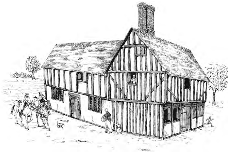
A reconstructed view of the timber-framed buildings which exist behind the brick cladding at Horner's Corner
