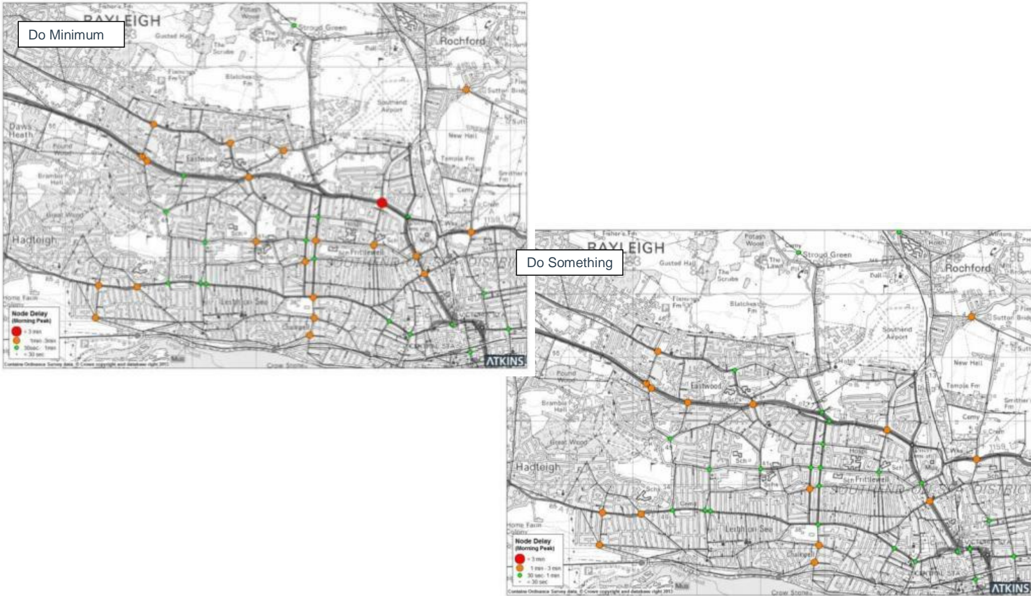
Figure 12. Highway Junction Delays Comparison AM Peak 2021
