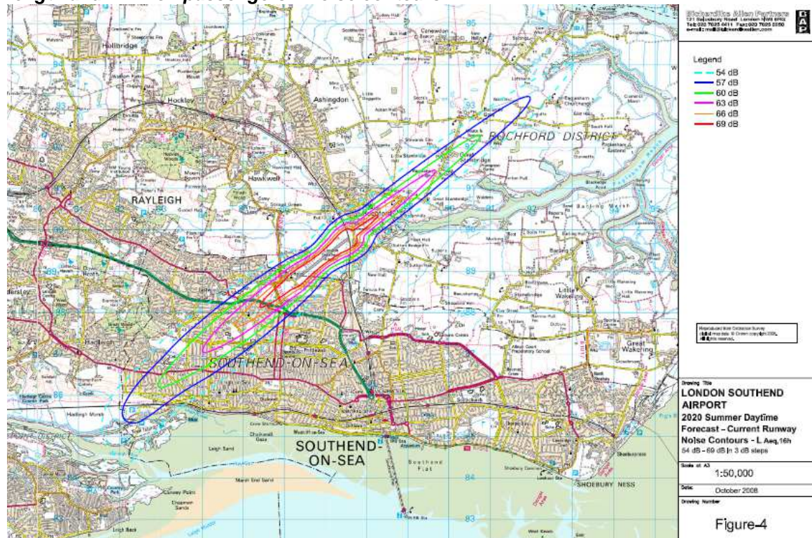
Figure 3.2: London Southend Airport 2020 summer daytime forecast at current runway length and 2million passengers – noise contours
