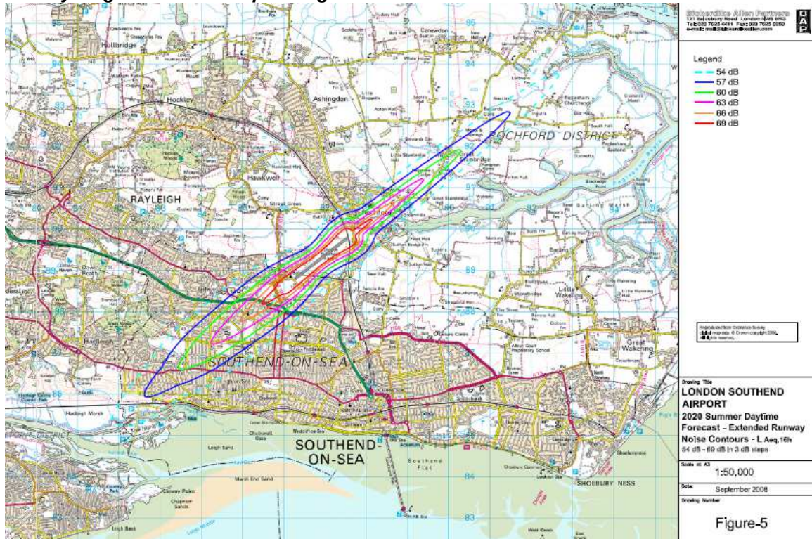
Figure 3.3: London Southend Airport 2020 summer daytime forecast at extended runway length and 2million passengers – noise contours
