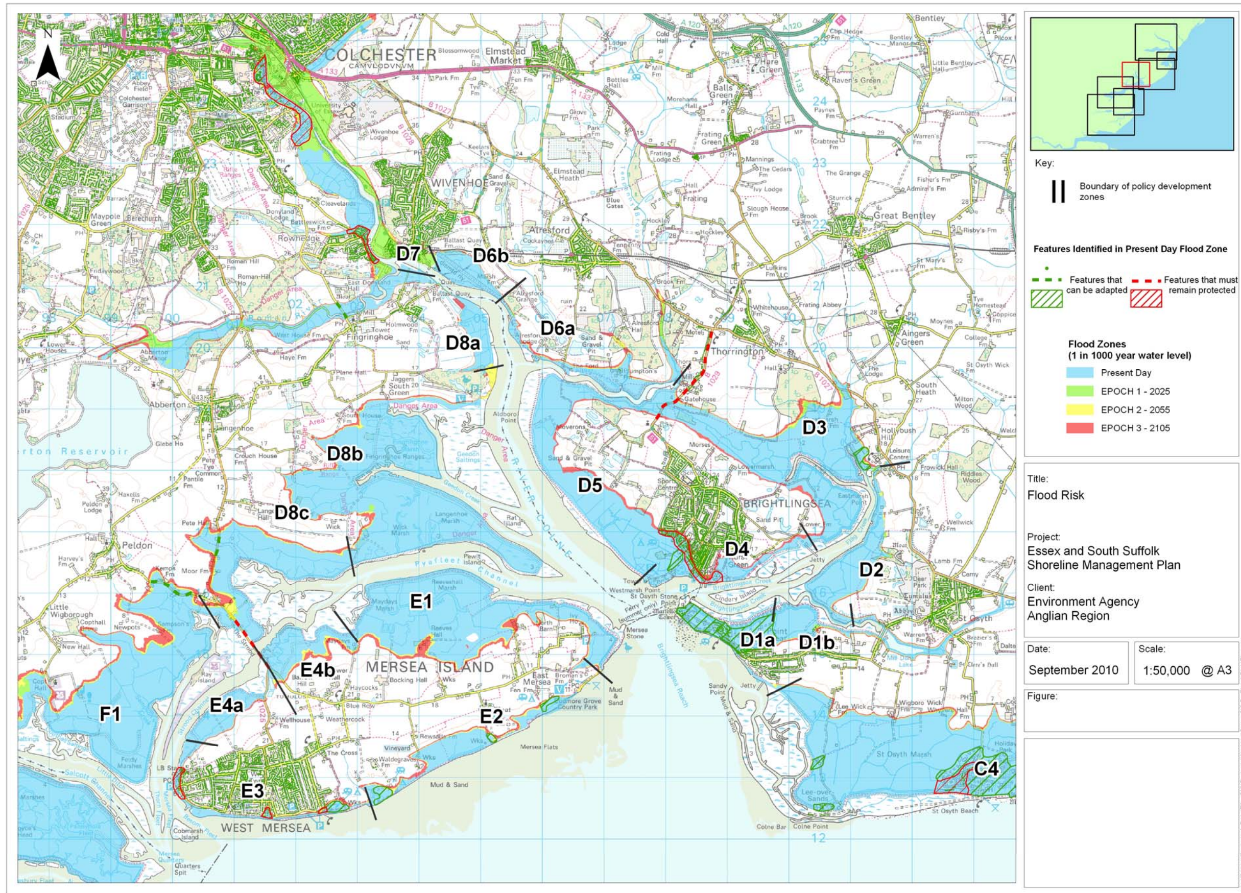
Figure 5-4 Flood Risk - Colne estuary and Mersea Island
